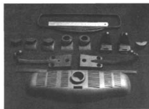
● 图1 用硅橡胶模具制造的汽车内饰件 Fig.1 The inner decoration components of automobile molded with silicone rubber tooling
