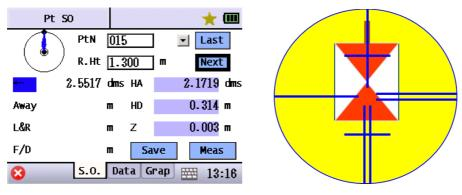
Click on Meas for measurement. The prism shall be moved forward or backward in the direction of view according to the prompt till Away value is displayed as 0 or close to 0. Fix points on the ground, and setting-out is completed.
