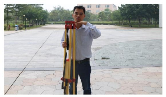
(2) Three feet of tripod are roughly equilateral triangle with length of side about 90cm. Not too short or too long. The proper length shall ensure your eyes slightly higher than the instrument eyepiece during observation.
